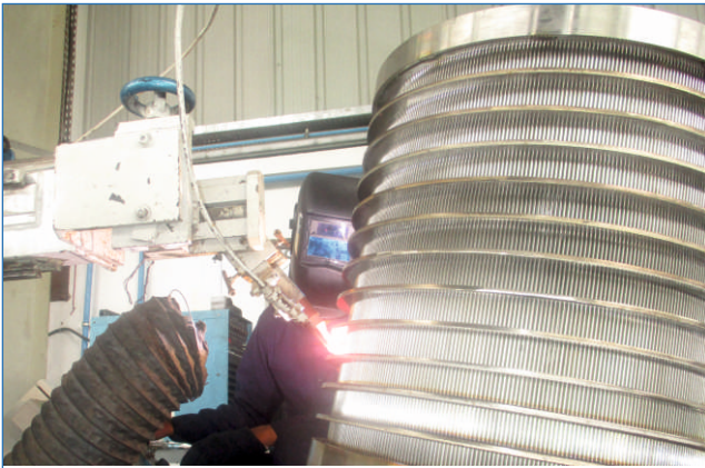
Automated welding machine
