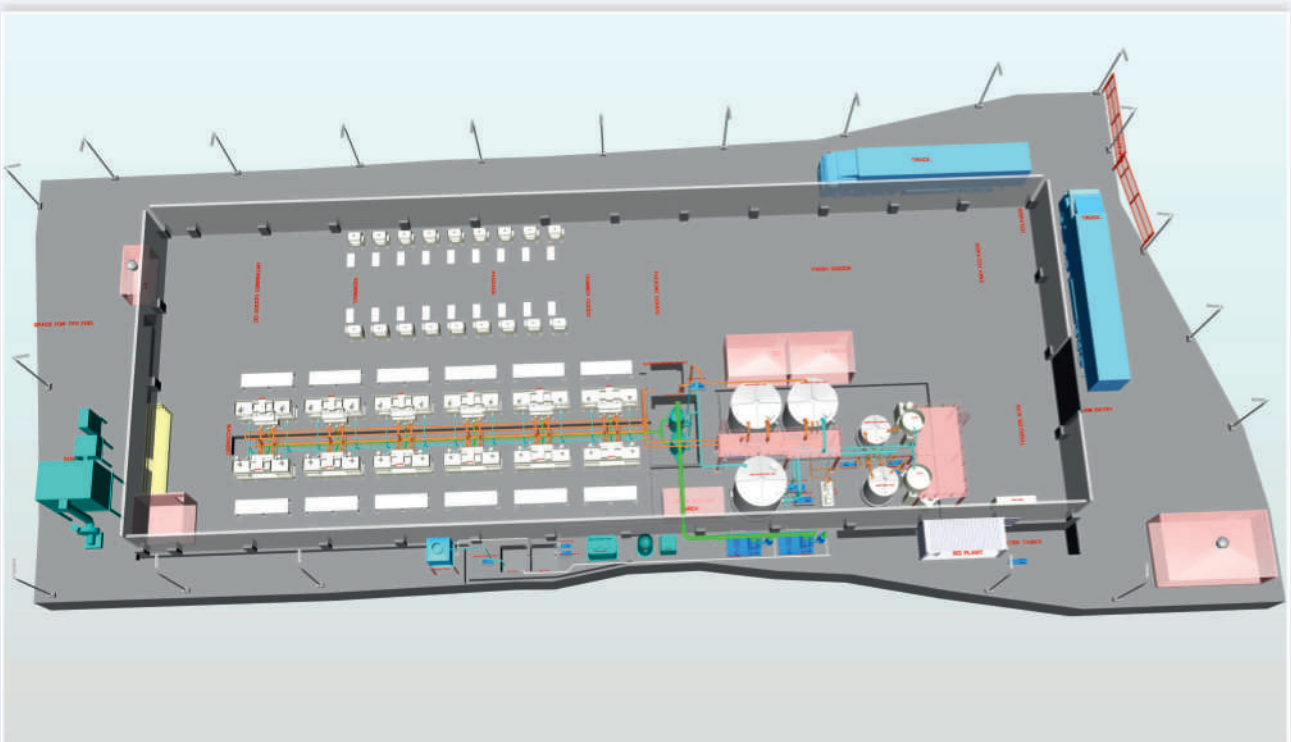
6TPD Molded Fiber Plant Layout
