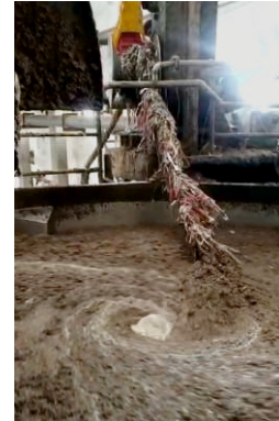
Parason Ragger removing contaminants from the pulp with Ragger Rope
