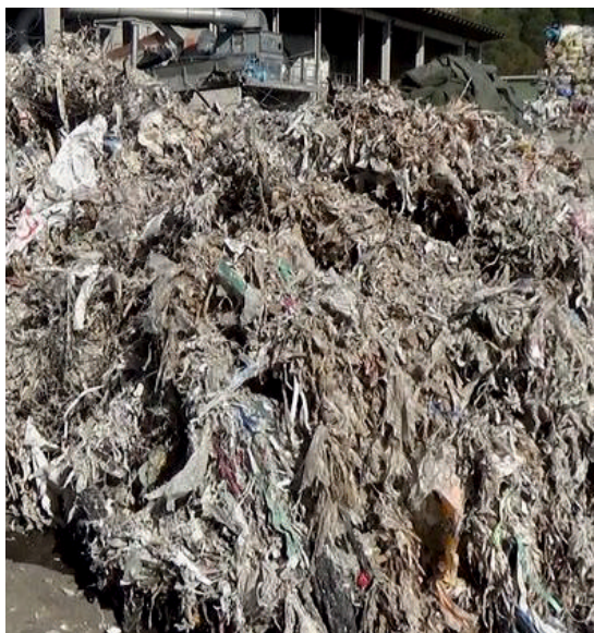
Contaminants discharged from pulper
